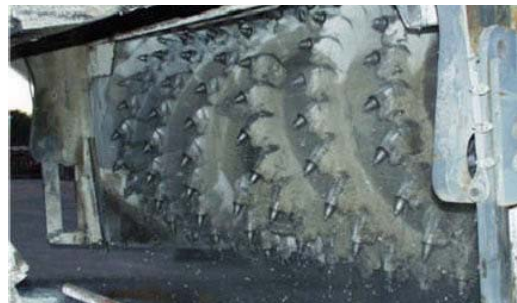
Cutting drum with enclosure on large milling machine.
