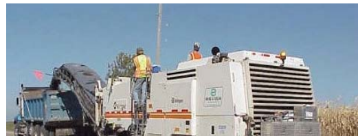
Cutting drum with enclosure on large milling machine.
