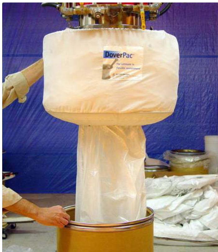
Figure 16. A continuous liner product off-loading system that uses a continuous feed of bag liners fitted to the process outlet to isolate and contain process emissions and product (Used with permission from ILC Dover.)
